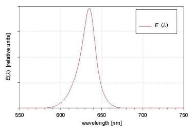
Figure 9 Optical output spectrum from the Aktilite CL128 lamp. The spectrum has a peak at 635nm with a FWHM of 18nm.
