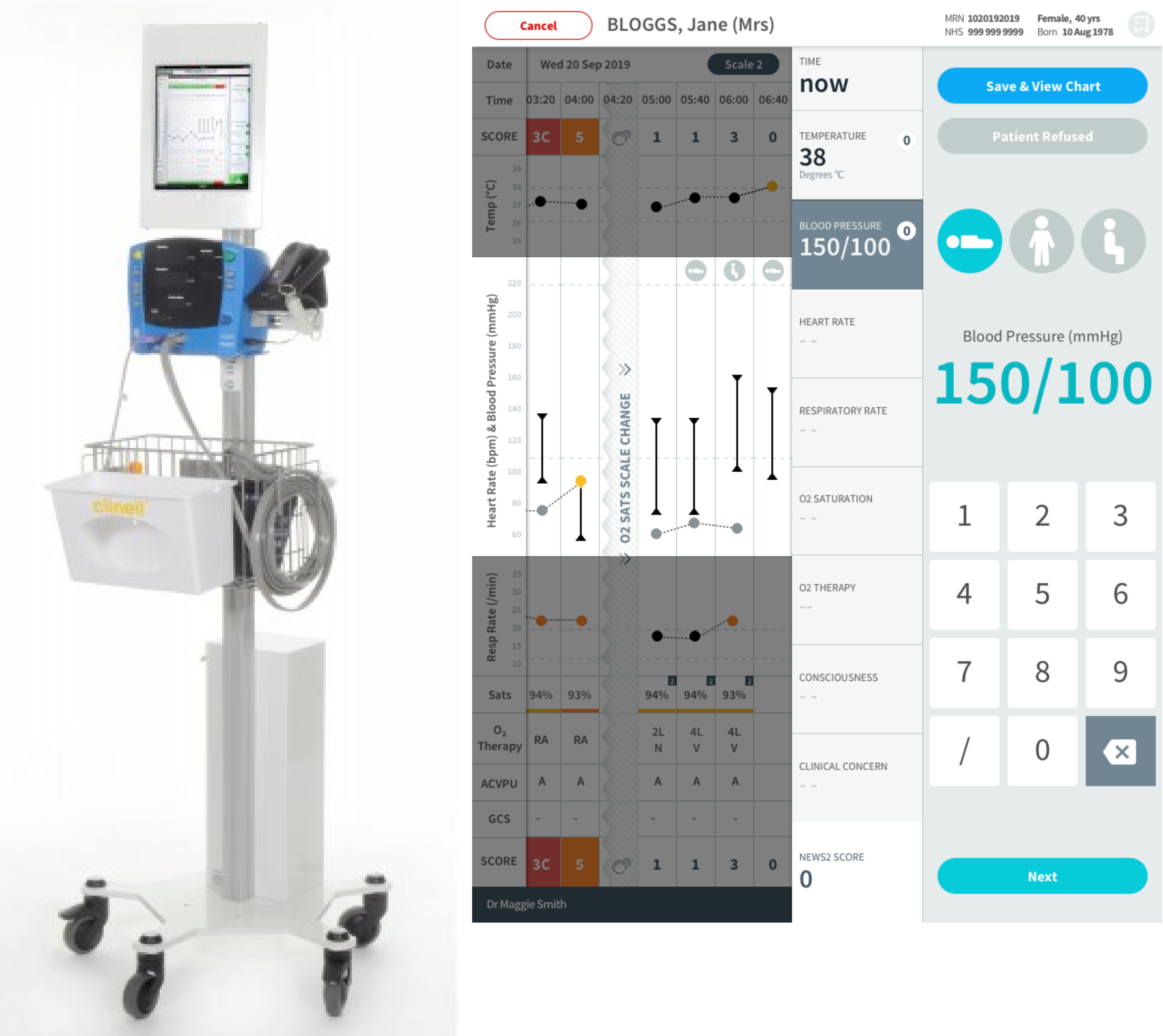
Figure 2: The SEND data entry hardware, and an example screenshot of the patient monitoring screen
