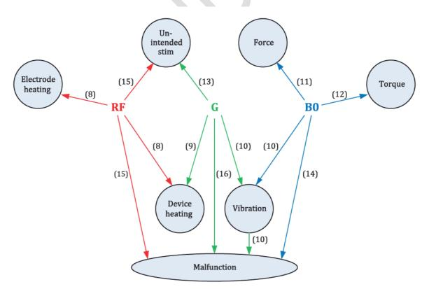
**Figure 2** Relationship between MR scanner output fields (RF, gradient, *B*0) and hazards (test method clause numbers in parentheses) according to ISO standards
