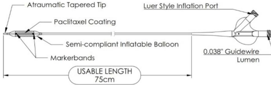
Figure 1. Optilume Drug Coated Balloon design (taken from company instructions for use)
