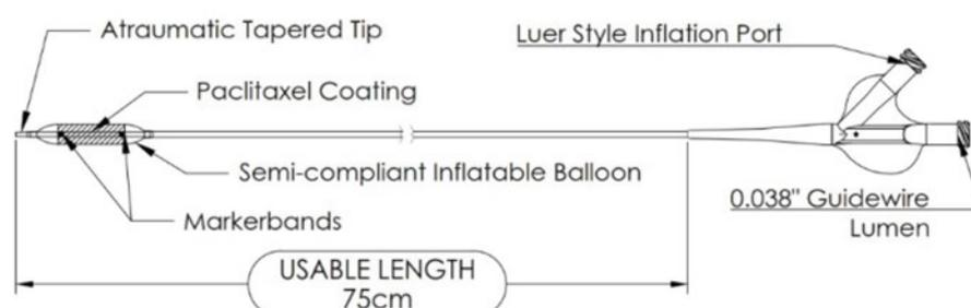
The innovative aspects that the Optilume device incorporates is the proprietary circumferential coating of  $3.5 \mu\text{g}/\text{mm}^2$  of the active pharmaceutical paclitaxel along
