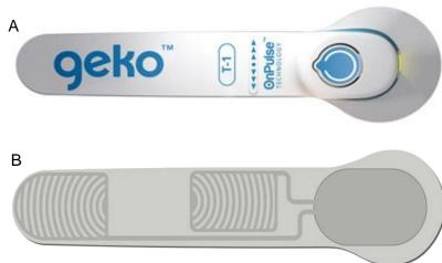
Key: A, top view; B, bottom view showing integral stimulator circuit and electrodes.
