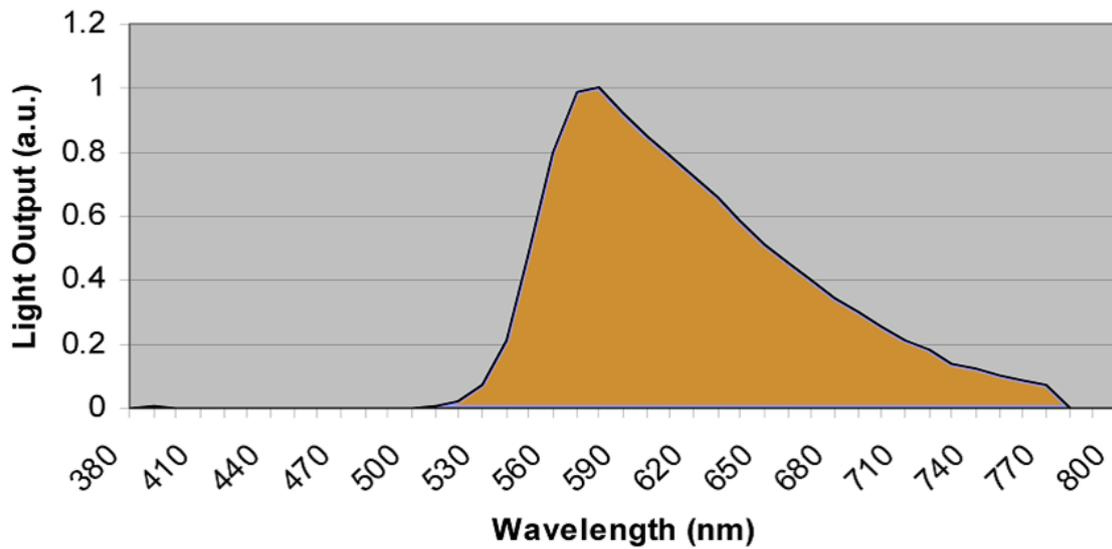
Figure 12 optical output spectrum from the portable PDT light source.
