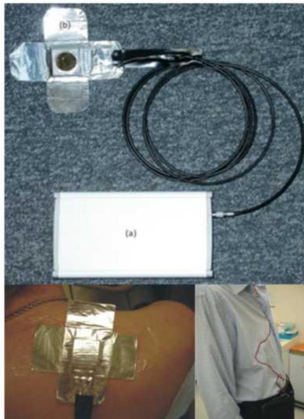
**Figure 11** photographs of the portable PDT light source showing, a) the two parts of the device, b) the light source attached to the patient, c) the power pack worn around the waist.
