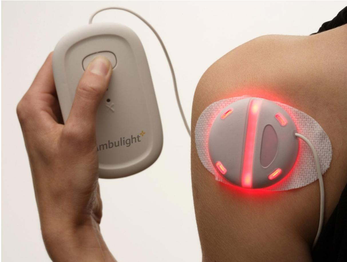
**Figure 6** Illustration of the Ambicare Health skin cancer plaster. The device comes in two parts; the first is the battery pack that is worn on the belt and the second is the light emitting plaster.
