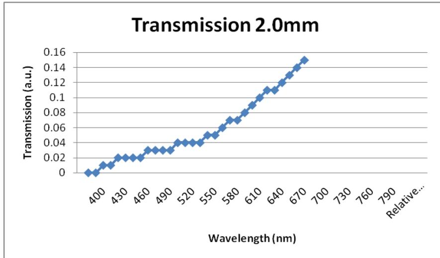
**Figure 2 Optical transmission spectrum for human skin at a depth of 2mm.**
