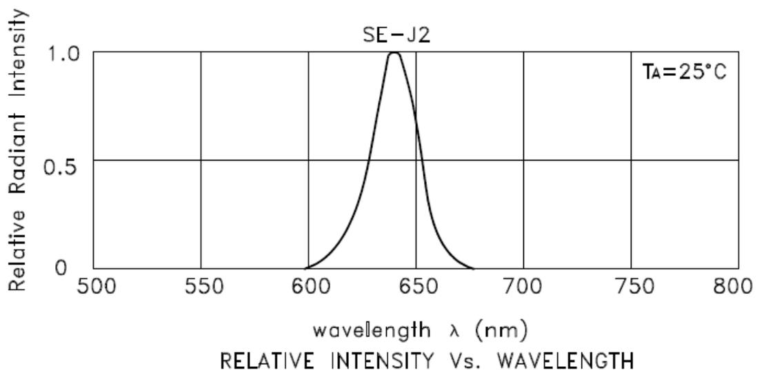
**Figure 7** Optical output spectrum of the LEDs used in the Ambicare Health light emitting plaster. The peak wavelength is at 640nm with a FWHM of 25nm.
