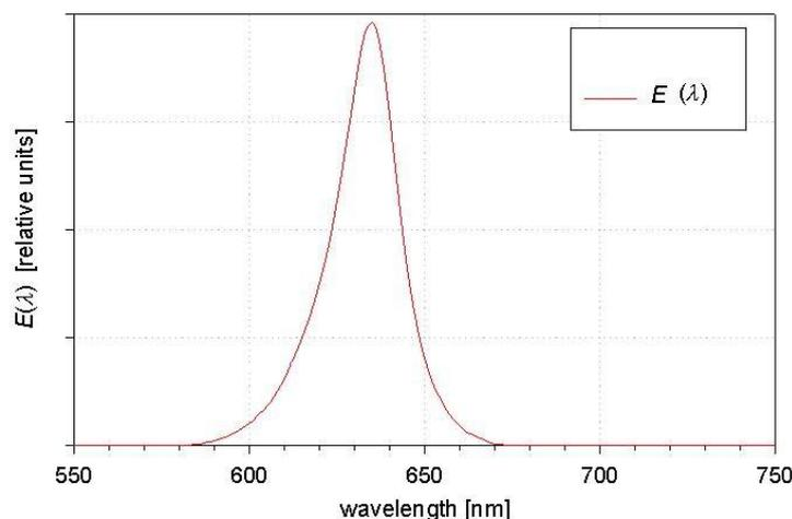
**Figure 9 Optical output spectrum from the Aktelite CL128 lamp. The spectrum has a peak at  $635 \text{ nm}$  with a FWHM of  $18 \text{ nm}$ .**
