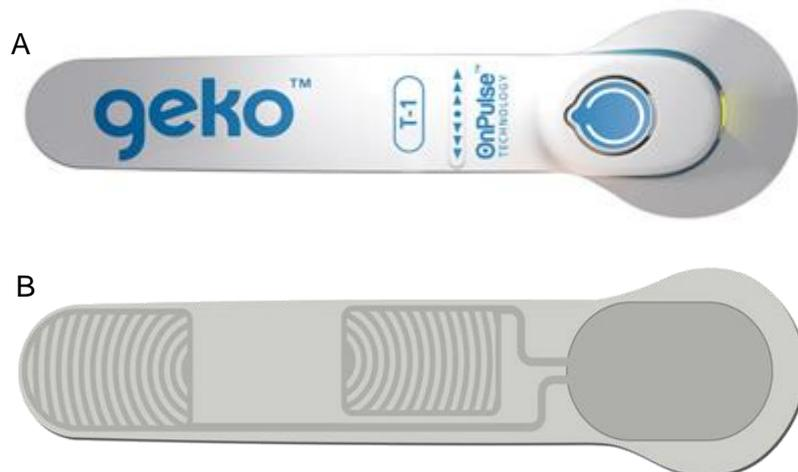
Key: A, top view; B, bottom view showing integral stimulator circuit and electrodes.
